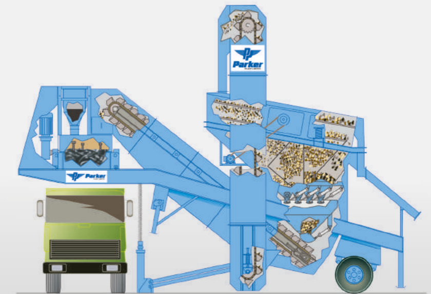
Material flow for a Super-BlackMobile 1500.
